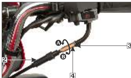
(2) Boot (3) Lock nut (4) Adjuster (A) Decrease free play (B) Increase free play
