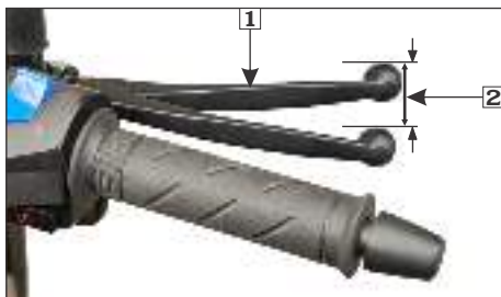
(1) Front brake lever (2) Free play 10-20 mm
