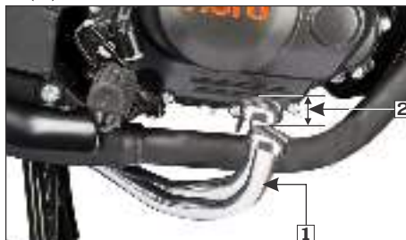
(1) Rear brake pedal (2) Free play 20-30 mm
